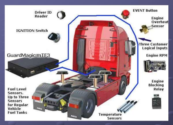
GuardMagic mTF module is established on a vehicle (can be done hidden installation) and in full automatic mode collect and store in the internal memory information about vehicle trip, movement parameters, fuel history, temperature history, data from additional sensors and electrical circuits.
