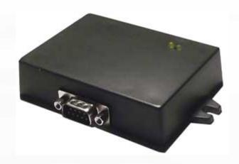
**GuardMagic DAFS** (DAFS1, DAFS2) receive voltage level ("analog" or "pulse-analog") from vehicle regular fuel level sensor and fix input signal to vehicle GND circuit.
