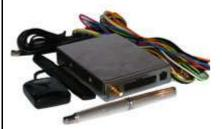
Simple GPS-GPRS vehicle module with fuel monitoring functionality (multi tank support). For On-Line Monitoring System (Vehicle fleet monitoring systems, AVL etc.). Universal communication protocol. Easy to installation and easy to use.
